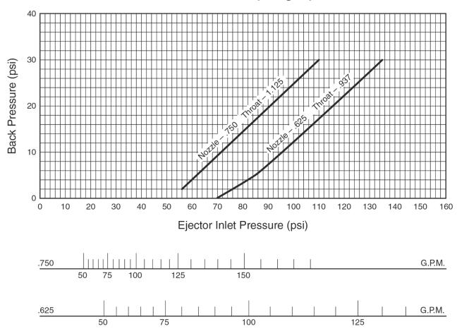
**Note:** Pressure combinations that plot below the line for any given nozzle are acceptable for operating that nozzle at the stated chemical feed rate for that chart. Pressure combinations that fall above the line for any given nozzle are not acceptable.
